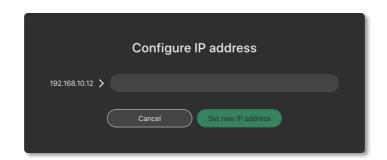
If the last octet of the new IP address is unchanged, the amplifier will show up on the workspace with the new IP. If not, it will show as offline on the workspace, and will show up as a newly discovered amplifier within the discovery list – it can then be replaced with the amplifier in the workspace using the standard method.
