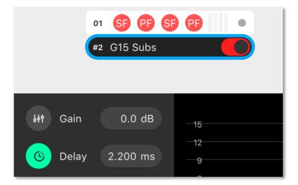
The Snapshot should now be stored on this amplifier, to enable offline recall from the Front Panel on site. Group Parameters (Gain / Delay / EQ etc.. can be adjusted from the Front Panel without use of the computer).
