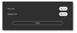
Pressing the (Lock) button to the right of the Display Lock text will toggle the display lock state of the relevant amplifier. An 'L' or 'Padlock' icon will be displayed on the amplifier LCD.
