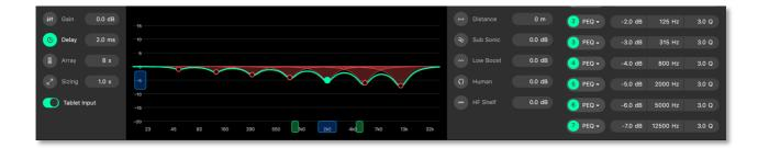
All group tuning parameters are enabled and disabled by clicking on the corresponding icon. A greyed-out icon means the parameter is disabled. A green icon means the parameter is enabled.
